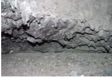
Fig. 2: Melting behaviour of castable from below right next to electrode hole.
